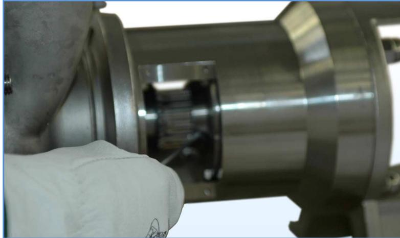
4. To facilitate alignment of the drive coupling manually rotate the shaft on the idle side;
