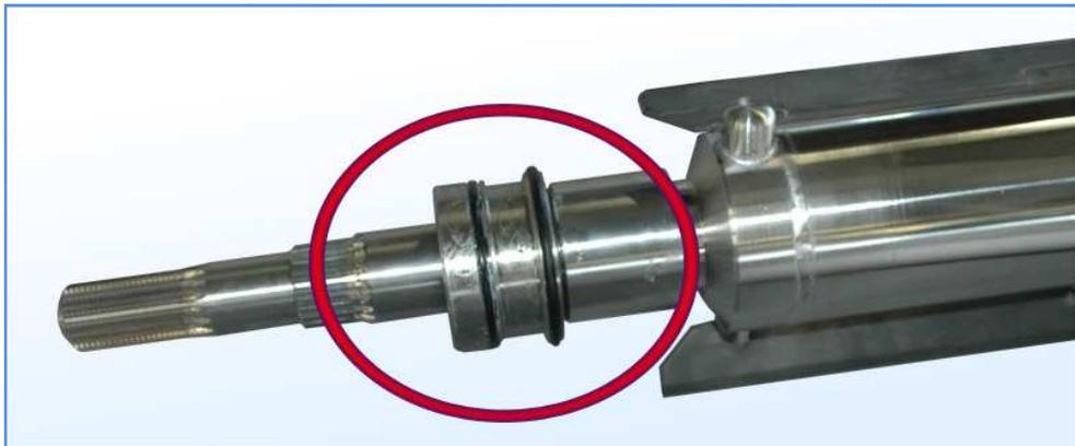
2. Gently insert the shaft ensuring that there are two sets of blades in contact with the exchange cylinder;
