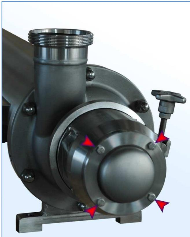
5. Loosen the safety device on the ring;
