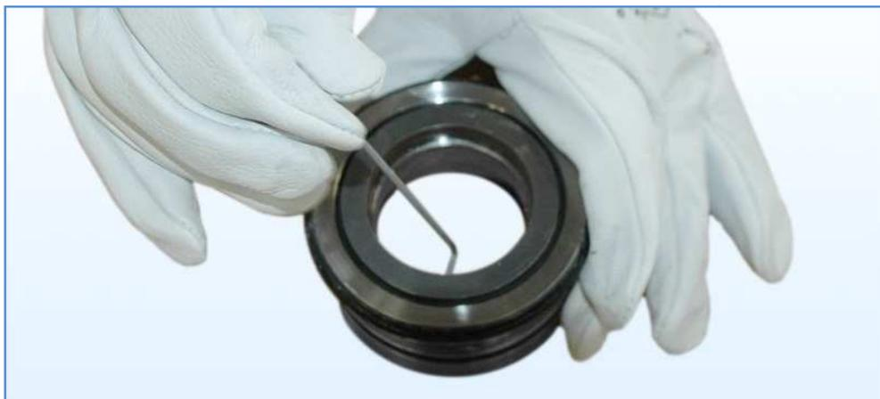
14. Fit the fixed walls of the new seals by pushing in all the way the ring and gasket, aligning the slot with the plug. **CAUTION: it is very important to avoid damaging, scratching, chipping the seal walls as this could affect machine operation.**
