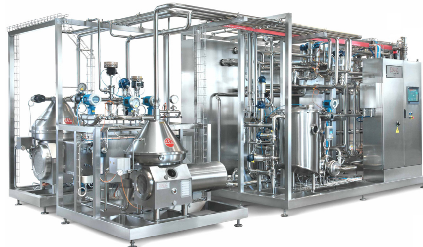
Whey pasteurizing line of 10 000 l/h with clarifier and skim separator
