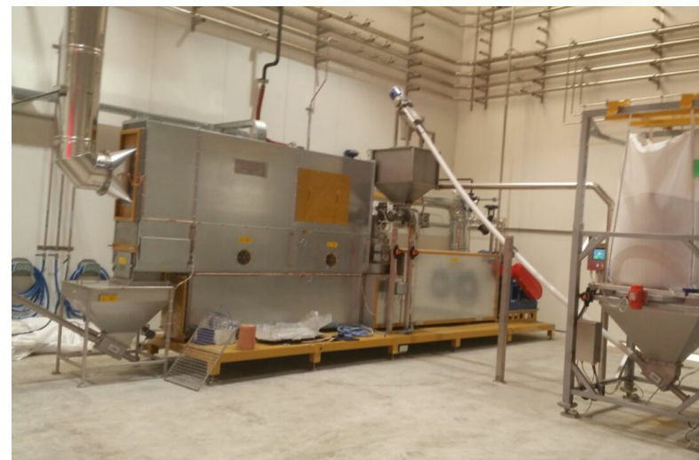
Roaster with hopper and flexible conveyor for bulk bag
